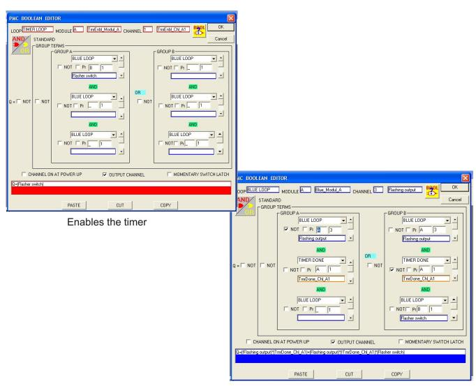
Latches the output on and off with each timer done pulse
