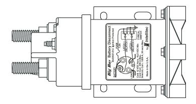
To close the Disconnect, a positive voltage is applied to the unmarked terminal of the coil and the negative of the supply is connected to the "S" terminal, for a brief period. When the power is removed, the relay is latched in the "on" or closed position. Current can now flow through the large terminals.
