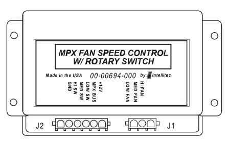
Note: The MONOPLEX Rear Fan Controller is a device used to switch power from the battery in a conversion van. Power from the battery should be connected to the controller through some type of approved circuit protection. Inadvertent shorts of the wires coming to or going out of the controller could result in damage and/or injury.
