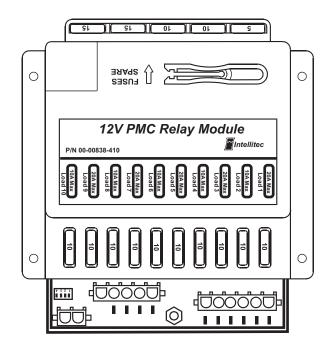
When using this module with PMC you should neither check the latched switch box in the Windows set up software for the pushbutton nor should a Boolean be written to operate the output. Channel P10 for 3 seconds will unlatch all latched outputs.
