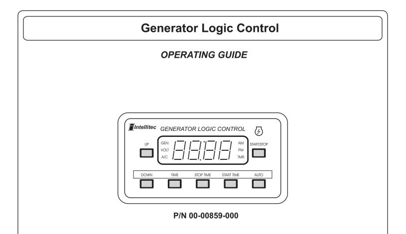
The Generator Logic Control (GLC) is designed to automatically start or stop a generator. Depending upon how the control is set, the Generator will start when either the battery voltage becomes too low, the air conditioner calls for cooling, or the time of day for auto-start has occurred. In addition to starting the generator, the control can be set to stop the generator at a specific time.
