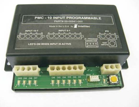
The approximate module dimensions are 7.25" X 4.75" X 2.25" (184mm X 121mm X 57mm).
