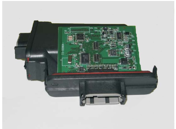
Dimensions of Module 5 1/4' x 4 1/2" x 1 3/8" (CANBus printed circuit board shown in photo)
