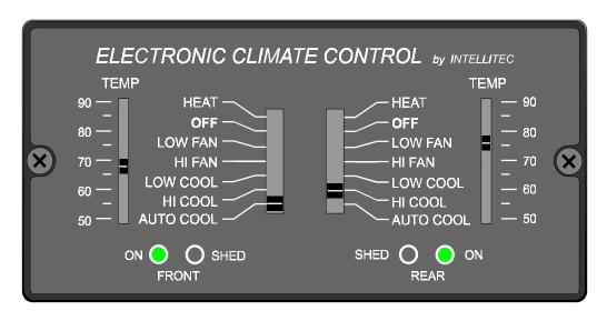
There are two identical sets of controls on the panel, one for each of the front and rear systems. The potentiometers allow the user to select a desired temperature for each system in the range of 50 to 90 degrees Fahrenheit. Moving the controls down, lowers the set point temperature. The two seven-position function switches are used to select the furnace's and air conditioners' operating modes. A brief description of each mode is as follows:
