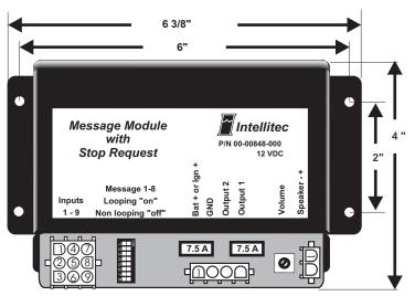
settings) and will have no effect on output 1. Output 2 will flash for several seconds each time input 1 or 2 is activated. Output 2 is intended to operate a driver's panel light, but may be used for any load up to 7.5Amps..
